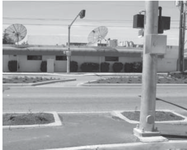
Mid-block crossing. Notice how median path directs pedestrians to look at oncoming traffic.
