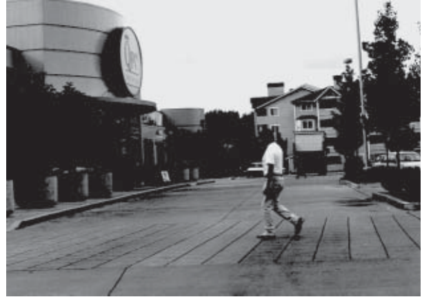
Pavement texture or scoring can be used to delineate the pedestrian travel area in a parking lot.
